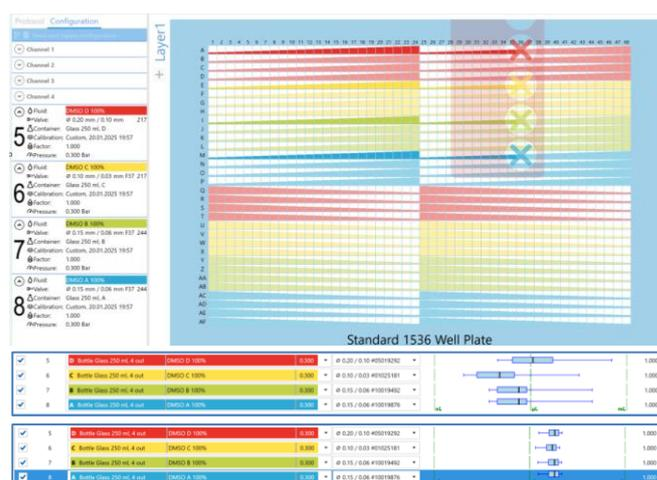
Figure 1 Dispensing Pattern and calibration range with factory calibration (water) and after LUMINA calibration.
