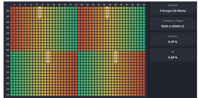
Figure 5 CV & ACC for CH5 at 5,3µl after Calibration with LUMINA
