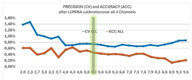
Graph 2 Graph 1 CV & ACC over all Channels & Volumes after Calibration with LUMINA
