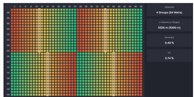
Figure 6 CV & ACC over all Channels at 5,3µl after Calibration with LUMINA
