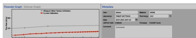
Figure 2 Calibration Curve with 24 support points
